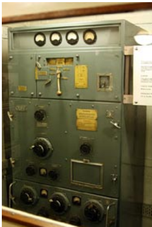
HF radio transmitter on HMS “Belfast”, type 603, medium power (400 W), for communications with aircrafts, ships and shore stations. Photo by Rémi Kaupp Källa Wikimedia Commons under GPL licens
